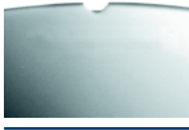
Fig. 2: A magnified view of a wafer notch as seen through the Nomarski Viewing System
